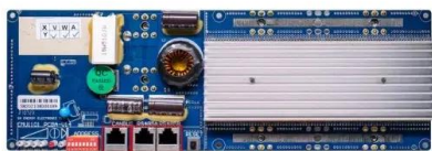
RS485 * Communication between battery and inverter Board size: 100x70mm RS485 Interface * Communication between parallel packs or BMS and PC Board size: 100x70mm
