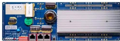
ES485 Communication between battery and inverter Baud rate:9600bps ES485 Interface Communication between parallel packs or BMS and PC Baud rate:9600bps
