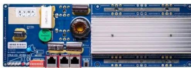
ES485 Communication between battery and inverter Band rate: 9600bps ES485 Interface Communication between power packs or BMS and PC Band rate: 9600bps
